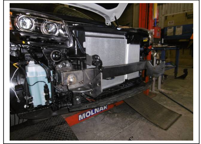
Figure 4. Steel mount fitted.
