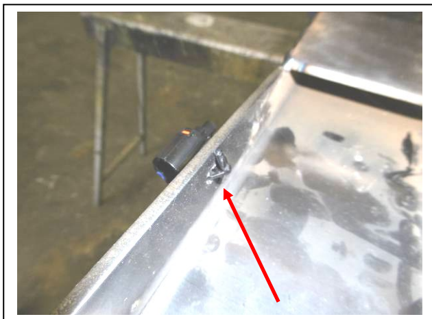
Figure 6B. Push plastic clip through hole so lugs protrude through.
