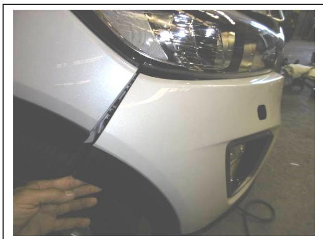
Figure 1. Pull out on rear wing to unclip away from guard and light.
